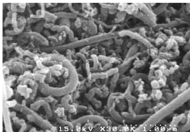
Figure 1. FESEM micrograph of the VGCNFs.
